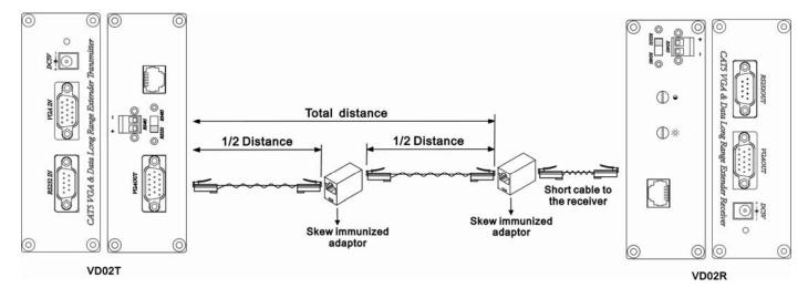
CAUTION: to avoid display equipment damaged, be sure to make correct cable connection and power for both VD02T before connecting VD02R
